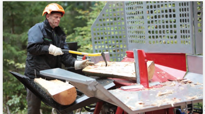
Logwood should be split as quickly as possible after harvesting for drying purposes. A variety of log splitters can be used for this.
