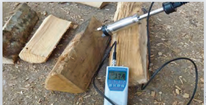
You can tell if the wood is dry enough for storage by measuring the moisture content.
